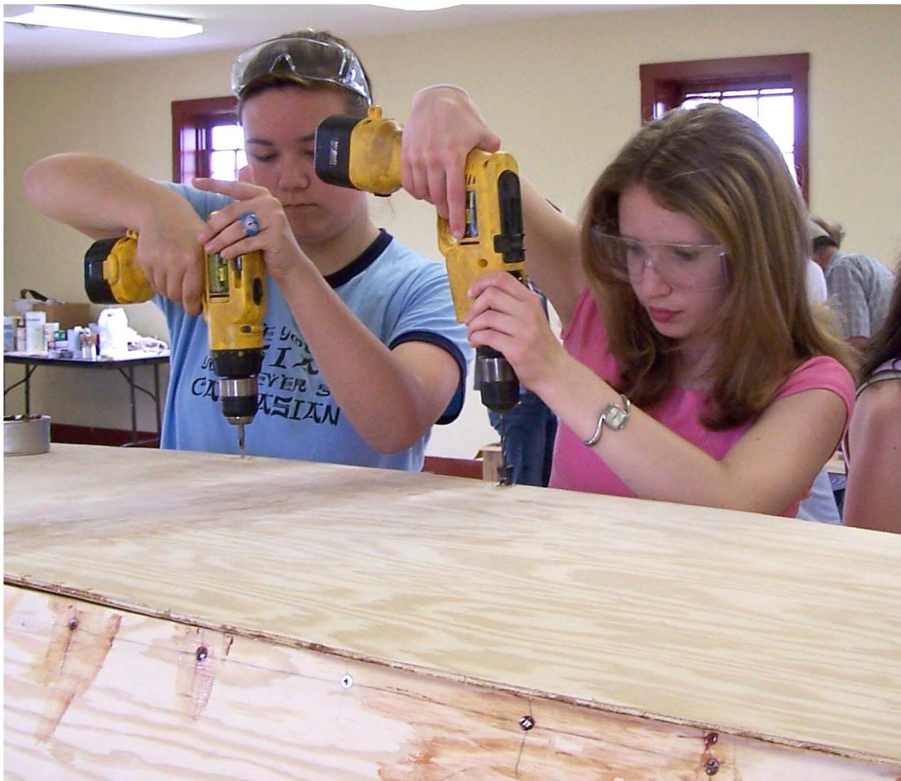
Rachael Carpenter, left, and Liz Bondelid work on attaching the bottom to their team's boat.
